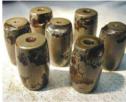
Rollers from a counterfeit spherical roller bearing
